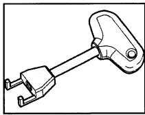
Puller T10094 - must be used to avoid damaging ignition coils during removal
