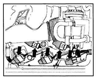
Disconnect connectors -arrows- from all ignition coils
