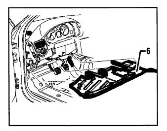
Unclip and remove lower cover -6- by sliding rearward out of clips
