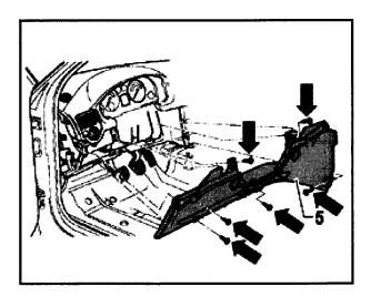
Remove (6) screws -arrows- and remove reinforcement -5-
