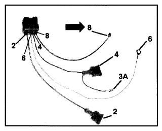
Locate terminal -8- (arrow) on the new wiring harness assembly
