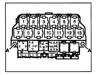
Reinstall relay carriers, secure with (2) nuts -Aand tighten to 2 Nm (18 in. lbs.)
