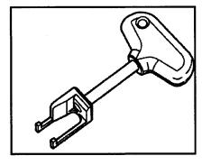
Puller T10095 - must be used to avoid damaging ignition coils during removal
