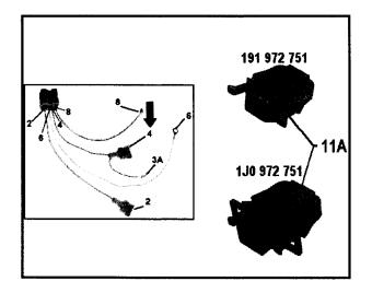
Insert this terminal -3- into connector housing -11A- (191 972 751 or 1J0 972 751)
