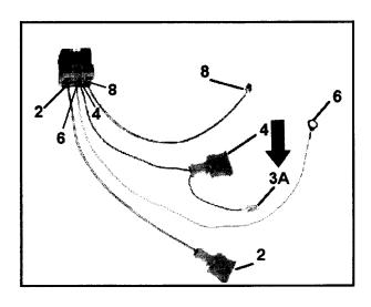
Locate terminal -3A- (arrow) [short wire from connector housing -4-] on new harness assembly
