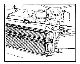
Remove lock carrier bolts -1- on left and right sides
