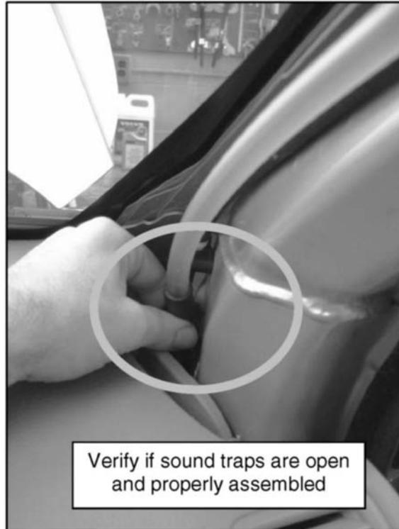
105. The Class Vehicles were manufactured with insufficient and undersized drainage openings in the sound traps.<sup>16</sup> This defect was prone to clogging of the sounds traps, thereby resulting in possible water ingress within the passenger compartment. Through TSB 83-34, Volvo instructs repair technicians to modify the sound traps of certain XC90 models by enlarging the opening in an
