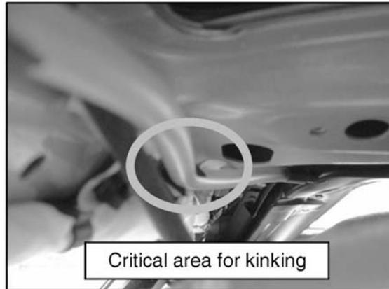
109. Volvo acknowledges the inferior quality of the sunroof drain tubes in TSB 83-34 by stating “[a] similar type of hose *with better rigidity than the original hose can be used to avoid kinking.* \* Semi-rigid Polyethylene tubing. Outer 1/2”, inner 3/8”. Manufacturer Watts (Part ref #42141525) *Available at Home Improvement Outlets or an automotive supply store.*”<sup>17</sup>
