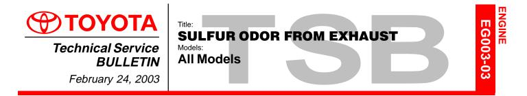
**Introduction** Some owners of Toyota vehicles may experience a sulfur–like or "rotten egg" odor from the exhaust system. Sulfur is a natural component of crude oil from which gasoline is refined and the amount of sulfur can be decreased through the refining process. The amount of sulfur in fuel sold in California is regulated, however gasoline sold in other states can have substantially higher sulfur content. Sulfur content also varies considerably between gasoline brands and locations.
