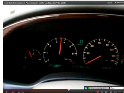
1:05 Tach oscillates between 3500 and 3900 RPM with no accelerator input.
