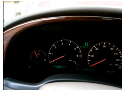
0:59 The engine shuts off after hitting the rev limit at 4000 RPM.
