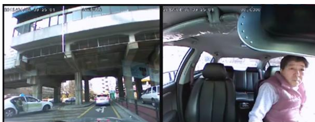
2:08 Releases hand brake to move up in line while feet are still outside the vehicle. Hears engine immediately rev to WOT. Passenger in another taxi also hears engine rev up.
