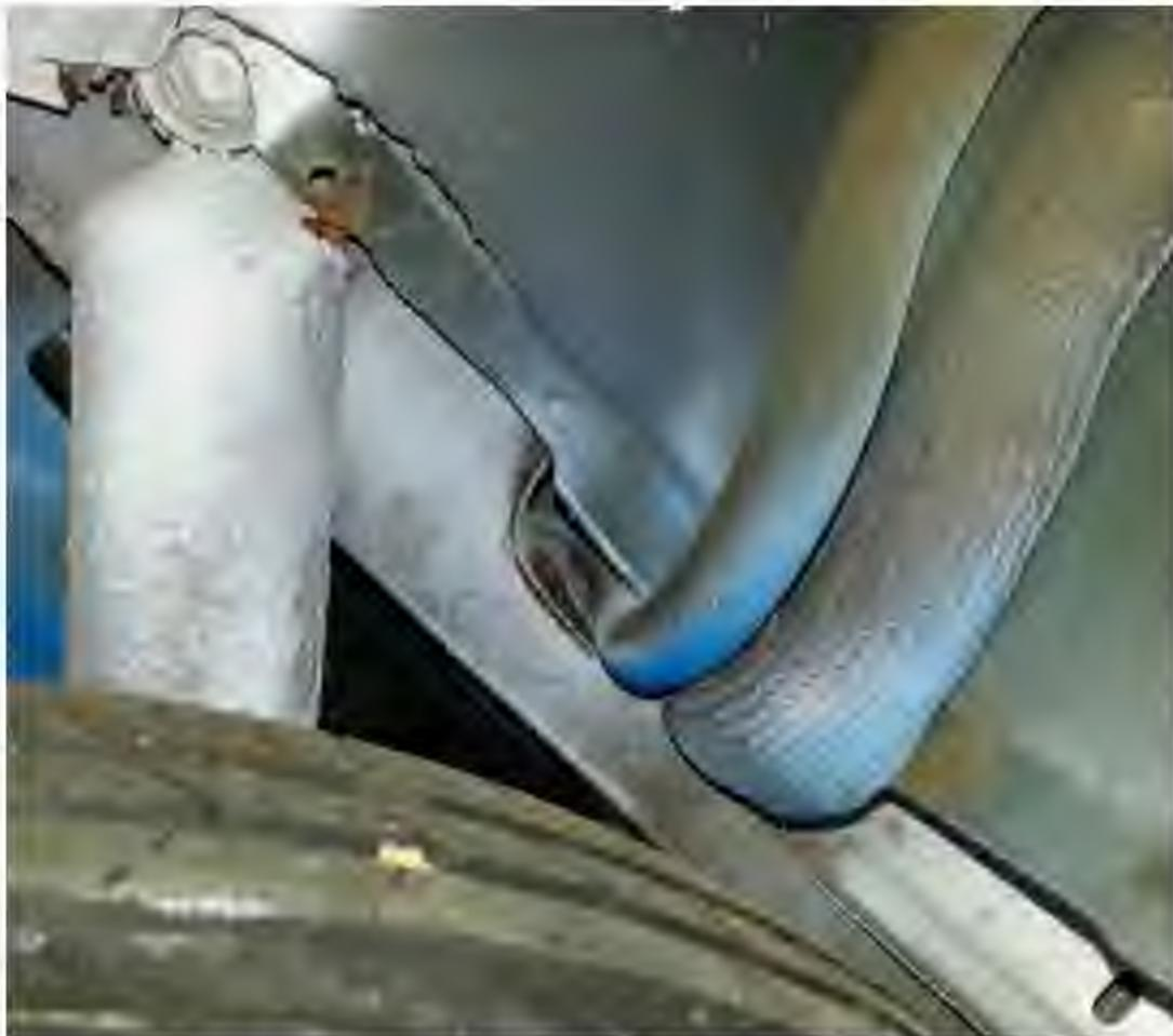
**Figure 16 Test#7 Rail with rust reinforced by hitch-receiver bracket, hose not cap tured – moderately rusted vehicle**
