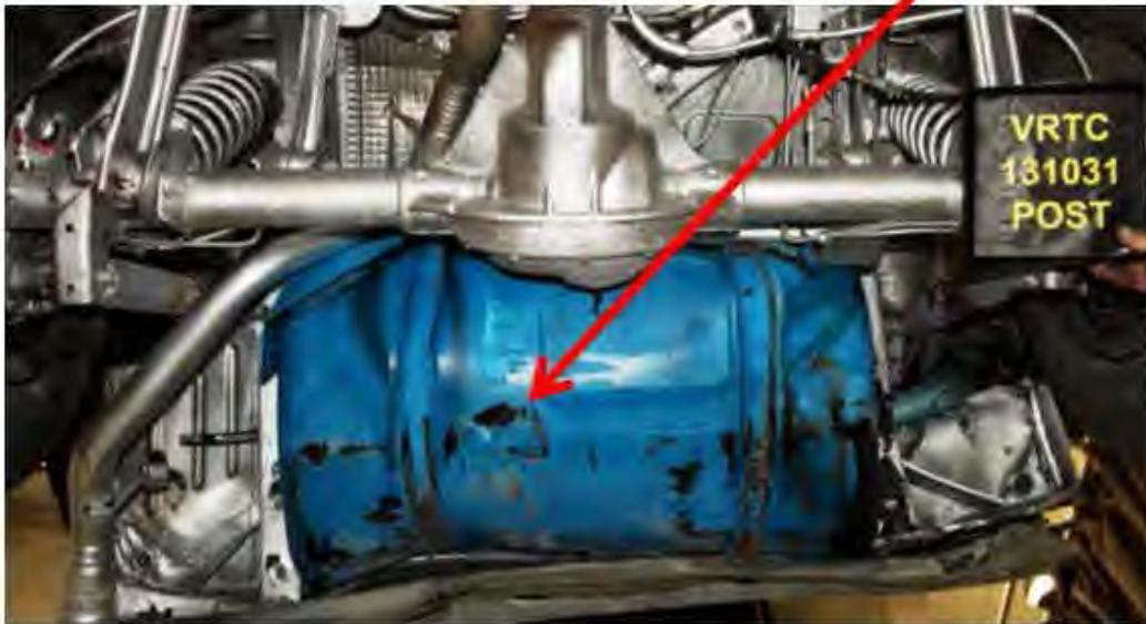
**Figure 21 – Post-test damage from Test #3 – No hitch-receiver**
