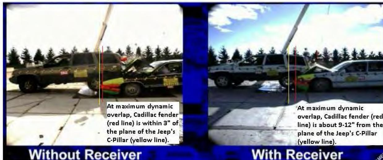
**Figure 14- Dynamic overlap between Cadillac and Jeep Grand Cherokee without and with a hitch-receiver**
