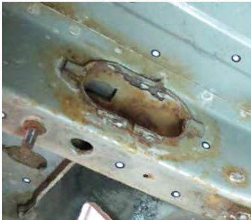
**Figure 11 - Frame rail relief tunnel for fuel filler hoses**
