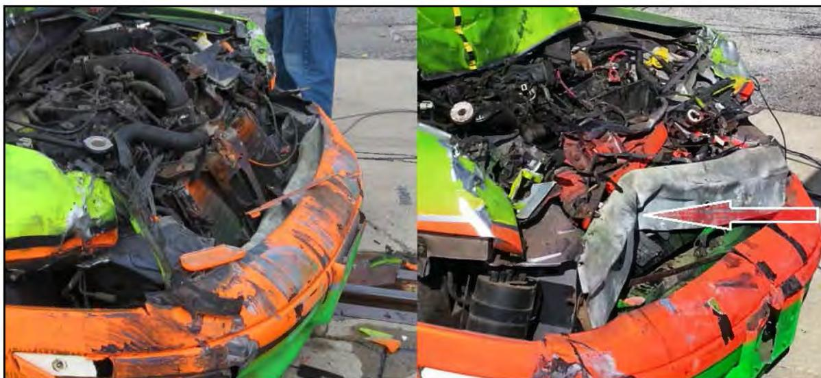
**Figure 7 - Neon bumper reinforcement Test 1 vs. Test 2. Arrow at hitch-receiver contact**
