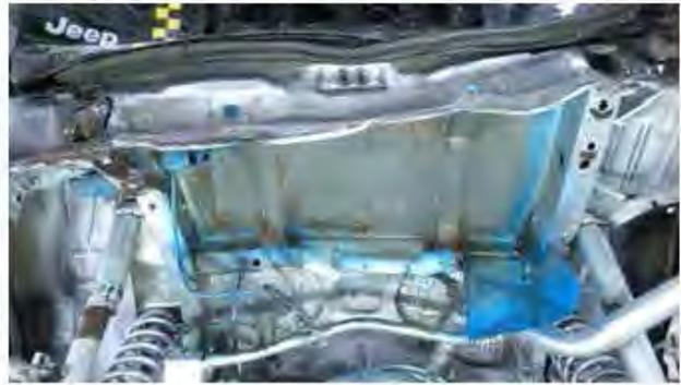
Fuel filler frame pass-through collapsed and pulled away from tank – Known source of leak from testing, Unknown if this occurred in the real-world crash
