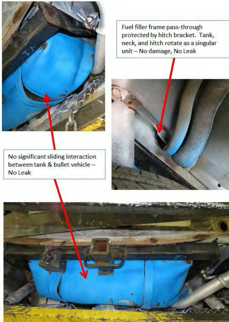
**Figure 22 - Post-test damage from Test #7 - With hitch-receiver**
