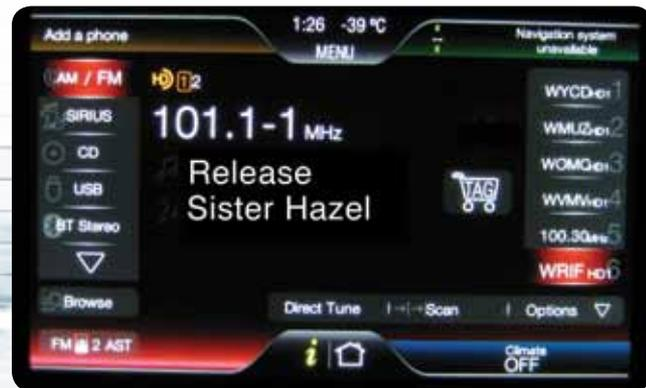
To access, press the lower-left corner of the touch screen. Then, press Radio > Options > HD Radio > On.
