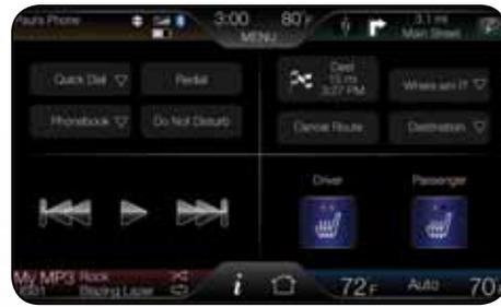
**Smart corners** home screen with frequently used controls displayed for easy access. The features contained here are based on the equipment in your vehicle, like heated and cooled seats, SD Card navigation map database or if you have paired and connected your Bluetooth®-enabled mobile phone.
