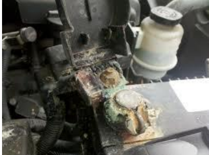
Fig 23. Corrosion on a battery terminal. Corrosion can also migrate 6 inches up the cable. 27
