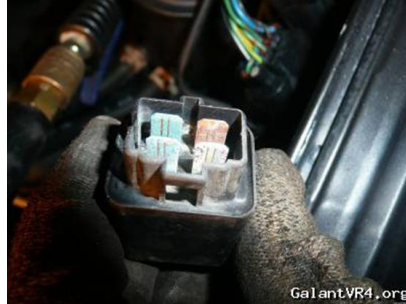
Fig 24. Corrosion in a radiator fan motor connector. 28
