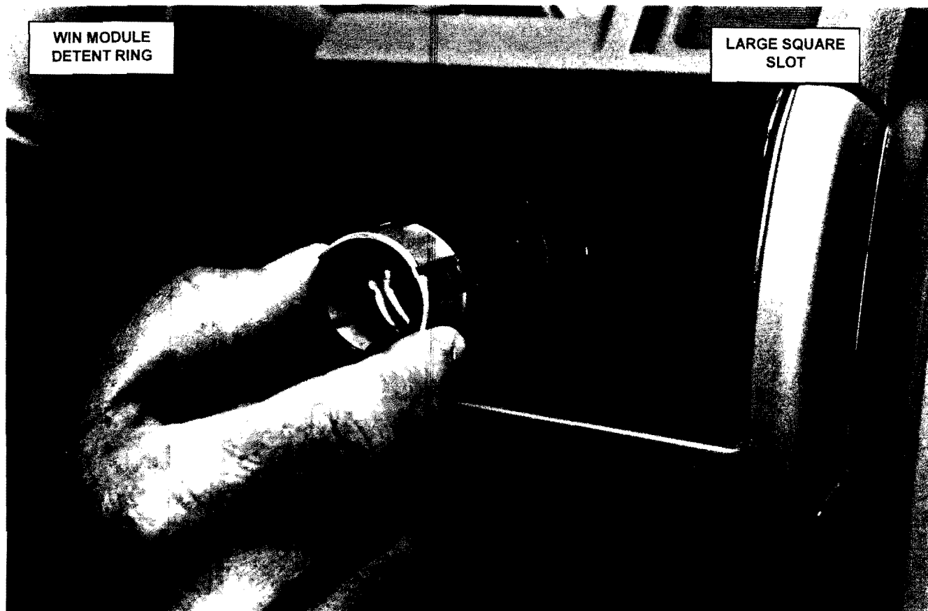
Figure 2 – Install WIN Module Detent Ring
