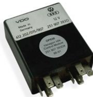
Figure A-5. Idle stabilizer electronics in its housing that fits under the driver side dashboard.
