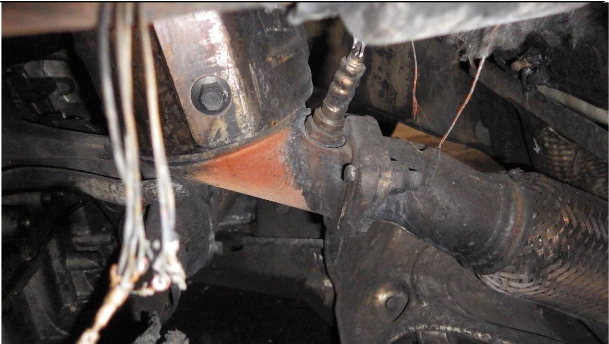
Figure 13: Hixon 2012 Kia Sorento, Exhaust near hole in rear of engine
