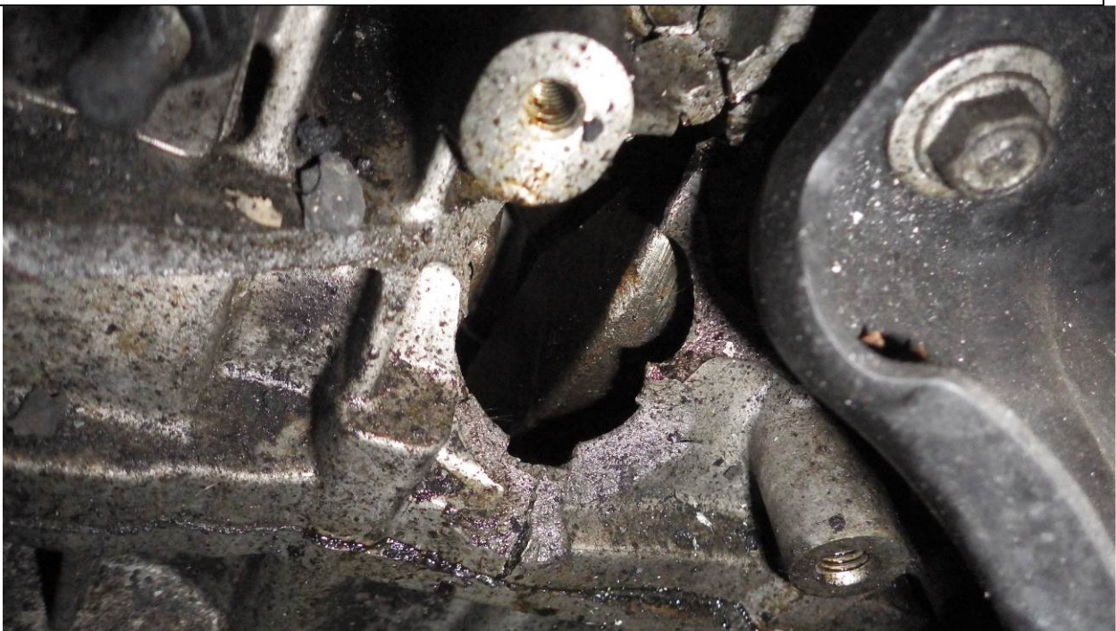
Figure 12: Hixon 2012 Kia Sorento, hole in rear of engine
