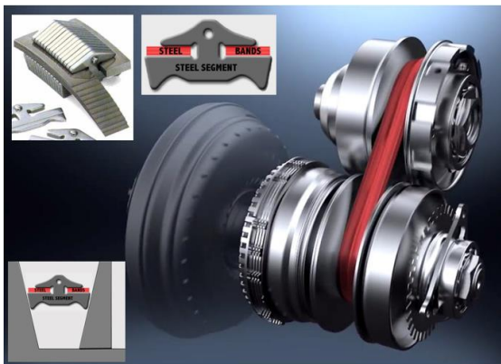
Fig 14. CVT transmissions use a steel belt to transfer torque from one pulley to another. The figure inserts show the Van Doorne belt design used in most Japanese vehicles. A chain link belt designed by LuK is used in most German vehicles.
