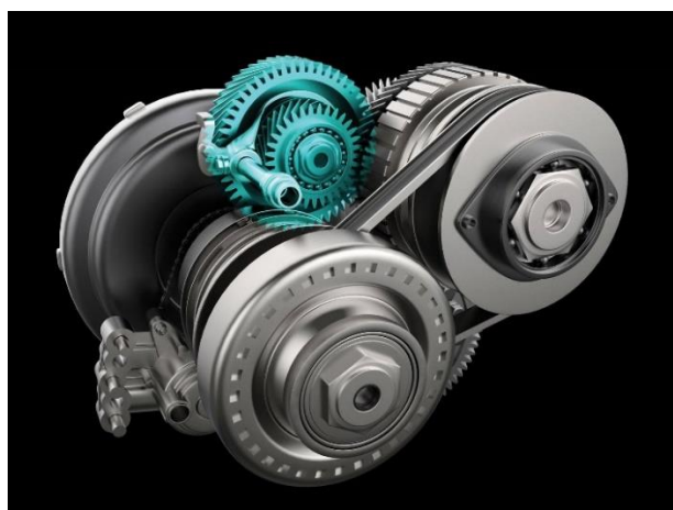
Fig 17. Toyota has added a fixed first gear to provide higher torque when launching the vehicle from a stop. Shifting into and out of first gear is done using a gear selector as found in manual synchromesh transmissions.
