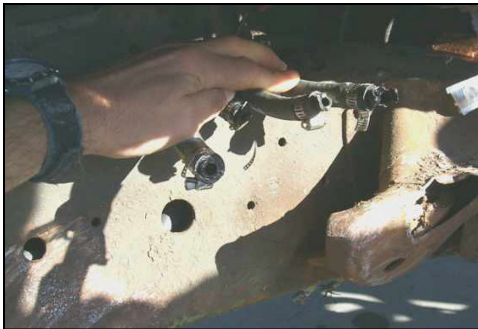
Figure 30: Fuel lines that were torn from the tank switching valve (test RP 01-036).
