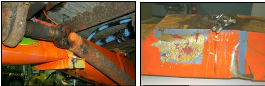
Figure 47: Denting caused by the drive shaft (test RP 01-038).
