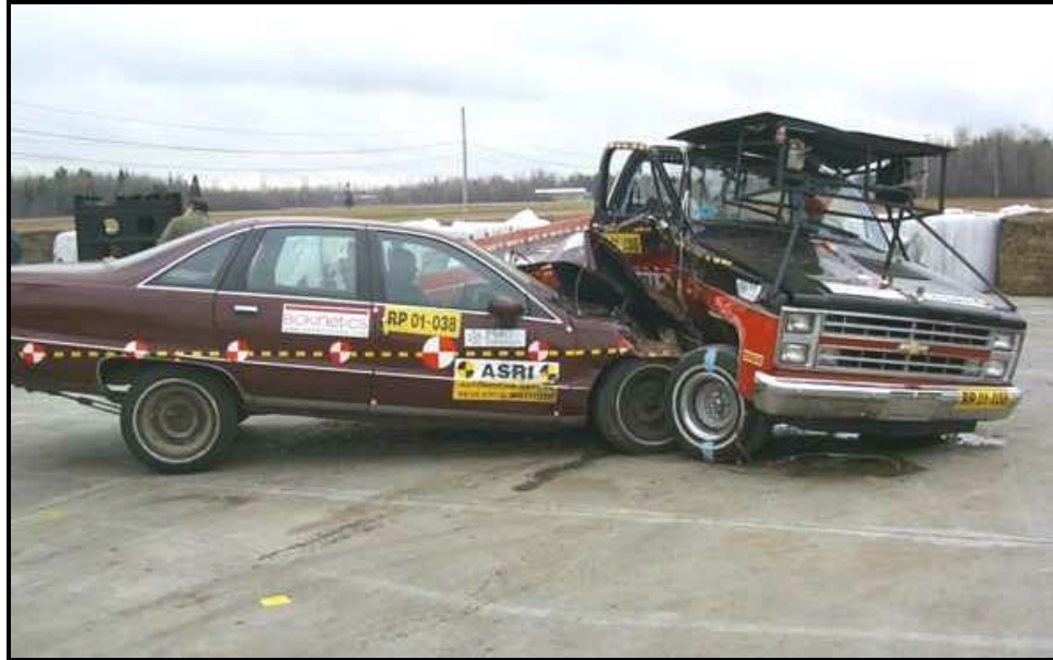
Figure 38: The final resting position of the truck and the bullet vehicle in test RP 01-038.
