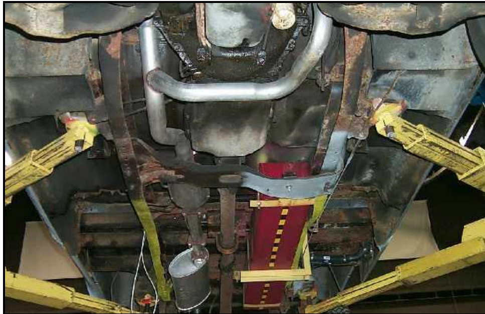
Figure 1: Location of the centre tank and the re-routed exhaust system in truck 2 (test RP 01-009).
