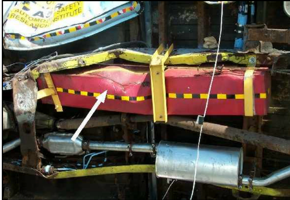
Figure 22: Denting to the fuel tank and damage to the tank mounting brackets (test RP 01-009).
