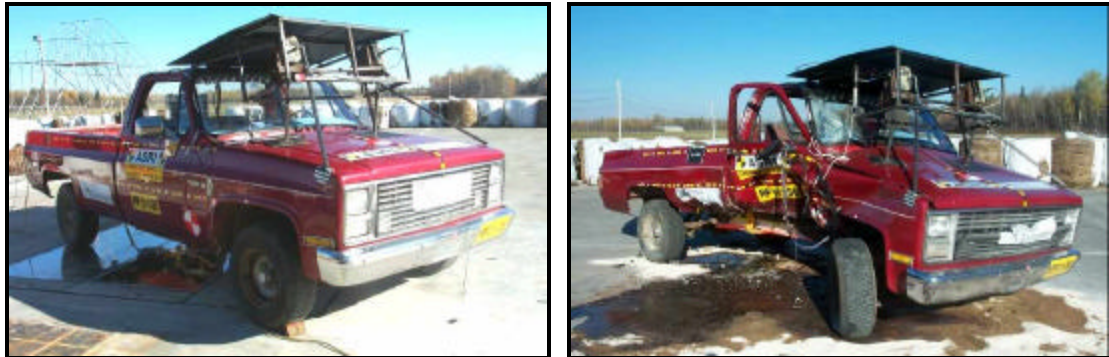
Figure 25: Pre and post test views of the GM pickup truck (test RP 01-036).
