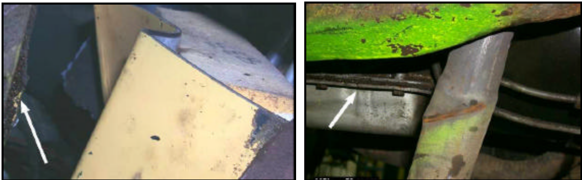
Figure 55: Damaged fuel line shield and exhaust manifold. The arrow is pointing to the edge of the transmission (test RP 01-039).
