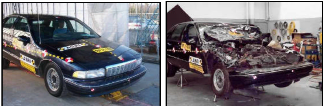
Figure 52: Pre and post test views of the Caprice bullet vehicle (test RP 01-039).
