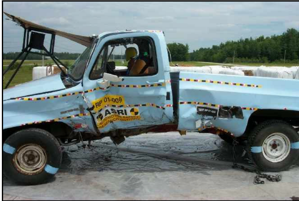
Figure 18: Damage to the truck (test RP 01-009).
