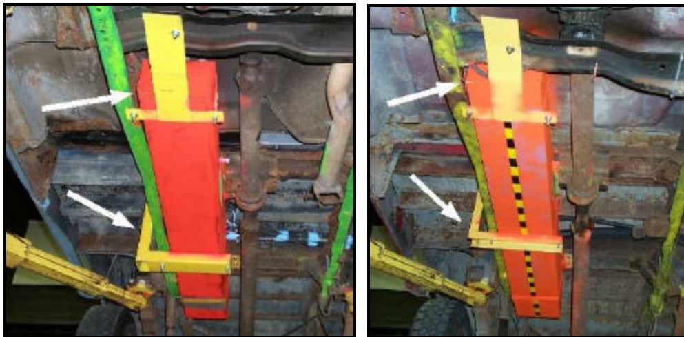
Figure 10: Rounded lower edge and tubular centre bracket on new centre tank used in test RP 01-039. Right photo is tank used in previous tests.
