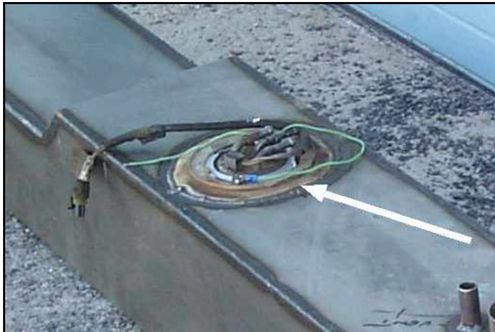
Figure 23: Sending unit seal where leakage occurred (test RP 01-009).
