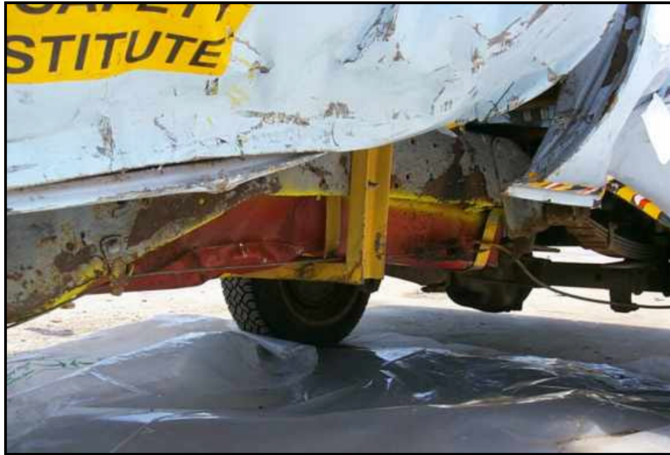
Figure 21: Tank mounting brackets following the test (test RP 01-009).
