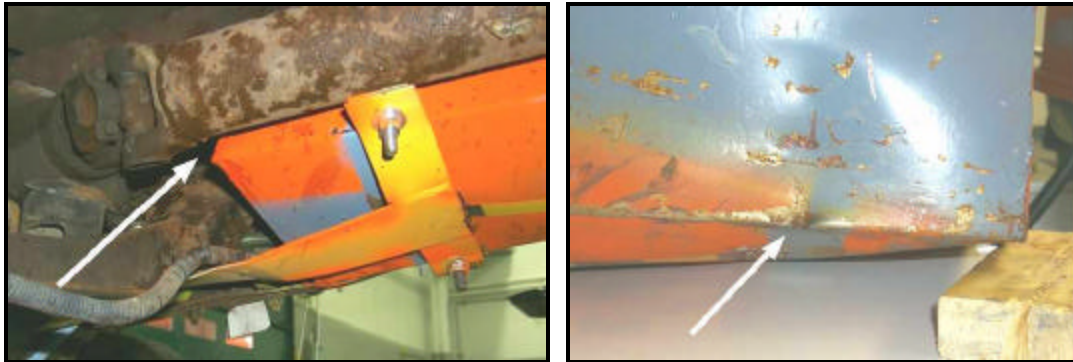
Figure 45: Damage to the front end of the tank front the drive shaft (left photo) and from the front mounting strap (right photo) (test RP 01-038).
