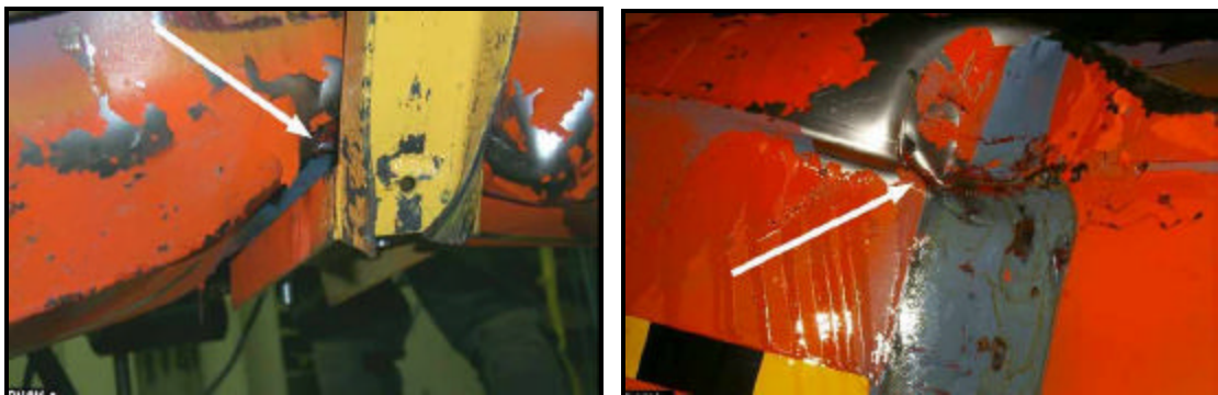
Figure 49: Hole in the tank behind the centre bracket (test RP 01-038).
