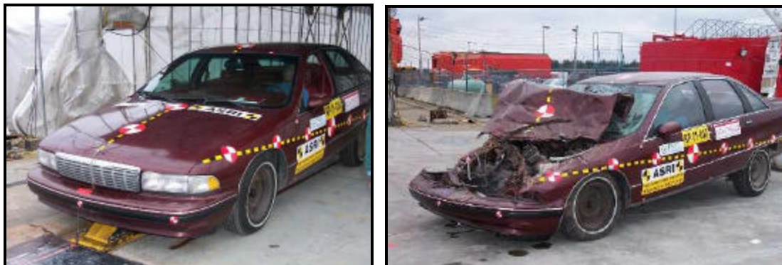
Figure 40: Pre and post test views of the Caprice bullet vehicle (test RP 01-038).
