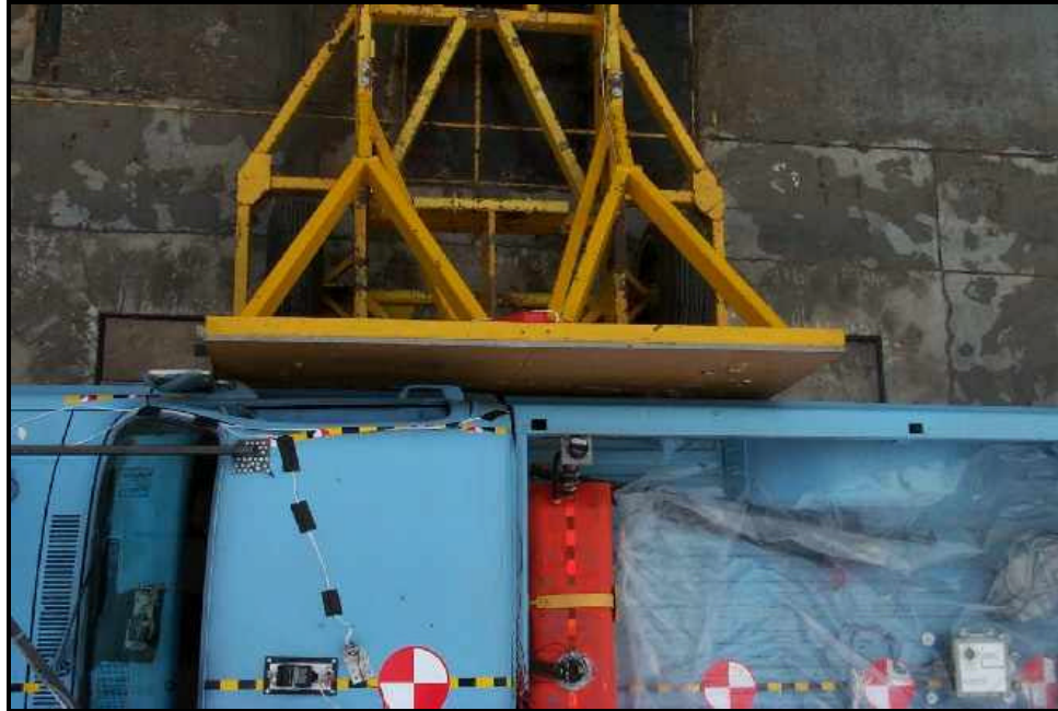
Figure 32: Over head view showing alignment of the barrier with the truck (test RP 01-037).
