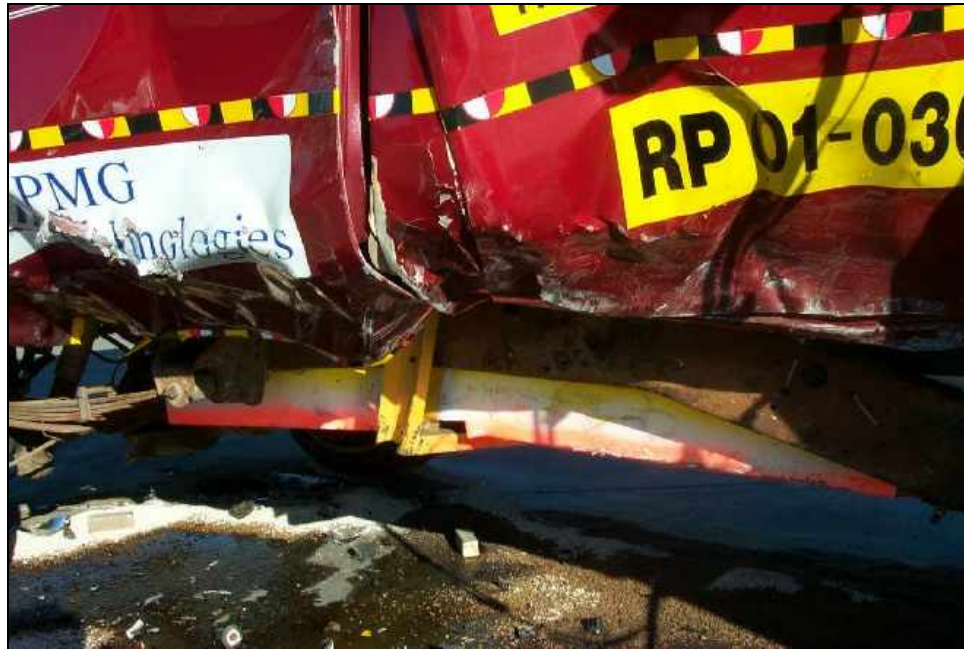
Figure 28: Plastic shield and centre mounting bracket. (Note: the rear bracket is concealed under the plastic shield.)
