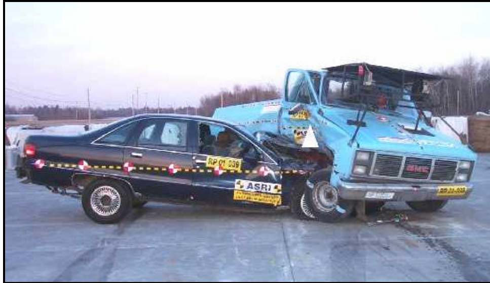
Figure 50: The final resting position of the truck and bullet vehicle in test RP 01-039.
