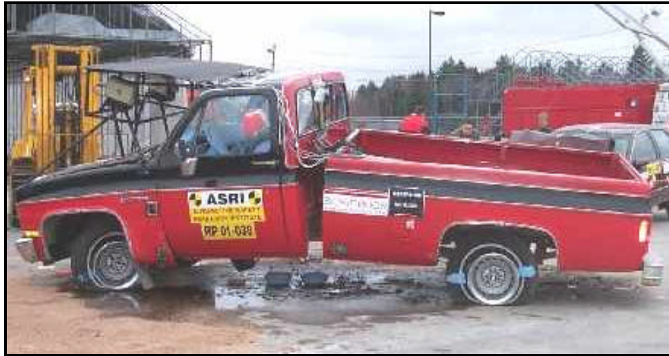
Figure 41: Far side tires were torn from their rims during the collision (test RP 01-038)
