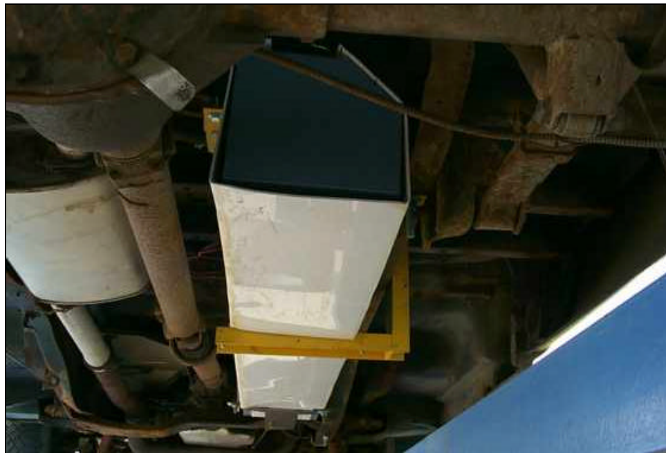
Figure 7: Rear view of centre mounted tank with the plastic shield covering bottom and both sides of the tank.
