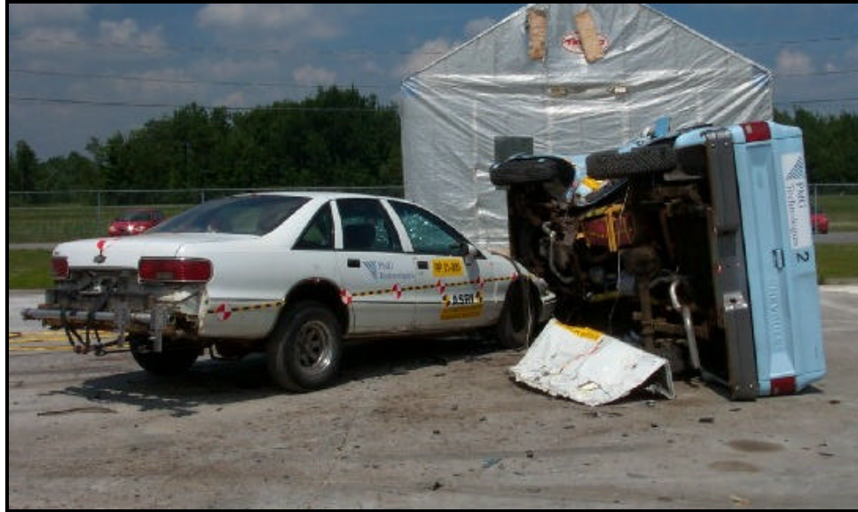
Figure 15: The final resting position of the truck and bullet vehicle in test RP 01-009.
