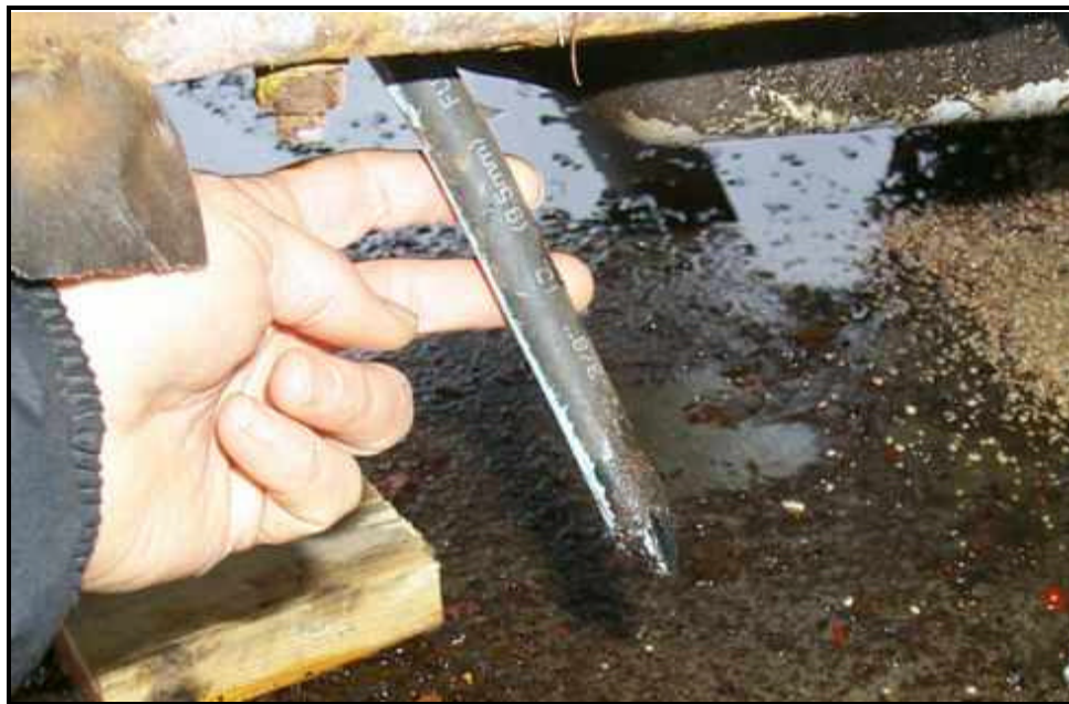
Figure 42: Severed fuel line (test RP 01-038).
