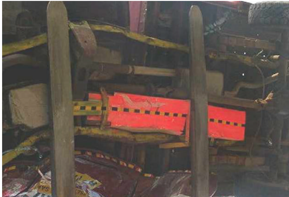
Figure 27: Centre tank and plastic shield following after the collision (test RP 01-036).
