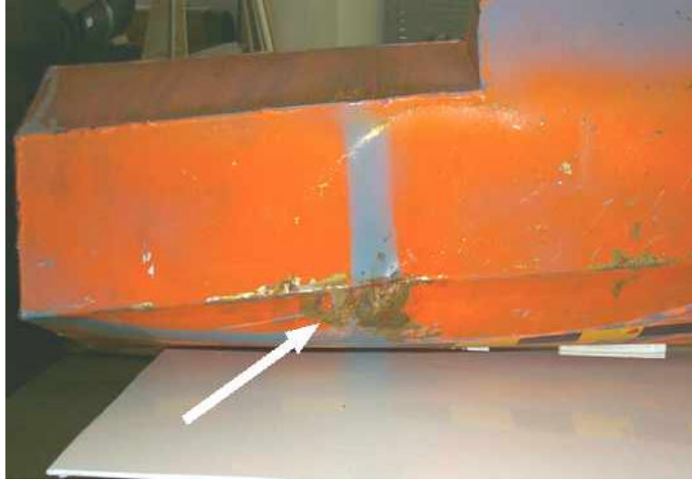
Figure 48: Minor denting caused by the rear mounting strap (test RP 01-038).
