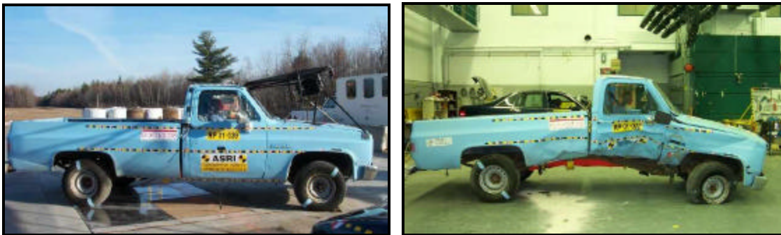
Figure 51: Pre and post test views of the GM pickup truck (test RP 01-039).
