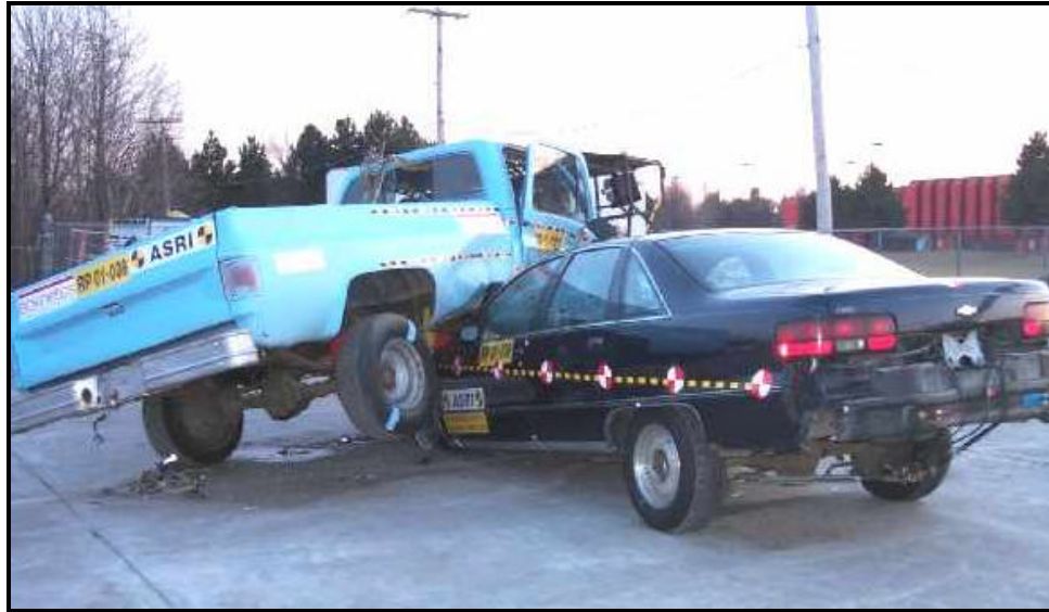
Figure 53: Post test view showing the right rear tire on the truck is noticeably off the ground (test RP 01-039).
