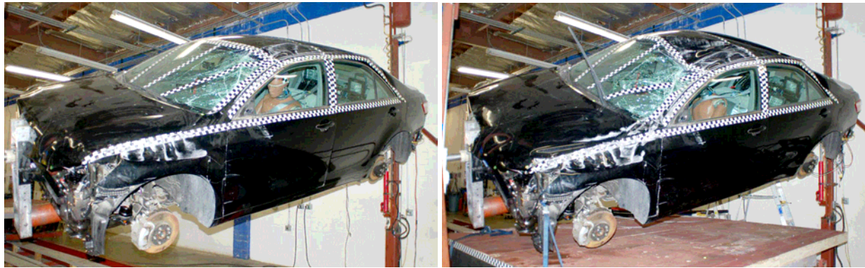
Figure 12. The 2007 Toyota Camry after the first roll JRS test (left) and the second.
