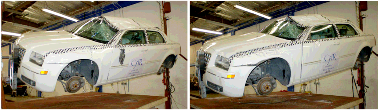
Figure 10. The 2007 Chrysler 300 after the first JRS roll test (left) and second roll.
