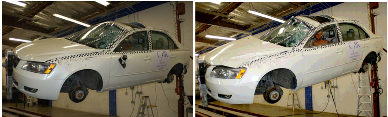
Figure 11. The 2006 Hyundai Sonata after the first JRS roll test (left) and second roll.
