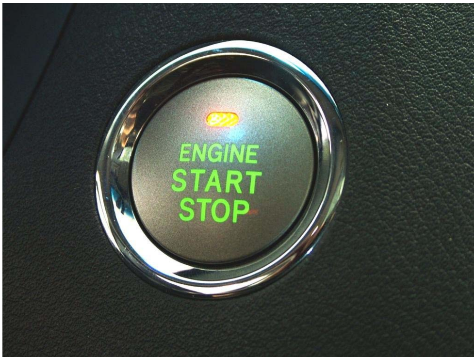
Figure 6 - Push Button Ignition Replaces Conventional Key
