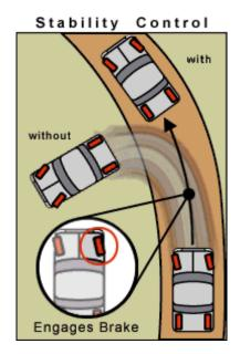
In an understeer situation, the ESC system gently applies the brakes of the inside rear wheel to help the front end follow the path of the curve. 12
