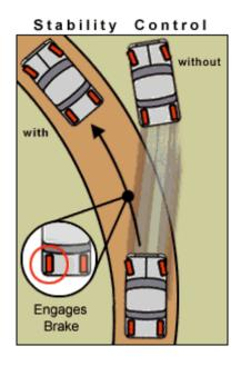
95. A non-functioning and/or damaged yaw sensor may impede or disable a vehicle's ESC system and prevent the automated adjustments needed to prevent an accident.
