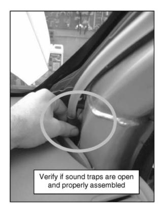
105. The Class Vehicles were manufactured with insufficient and undersized drainage openings in the sound traps.<sup>16</sup> This defect was prone to clogging of the sounds traps, thereby resulting in possible water ingress within the passenger compartment. Through TSB 83-34, Volvo instructs repair technicians to modify the sound traps of certain XC90 models by enlarging the opening in an
