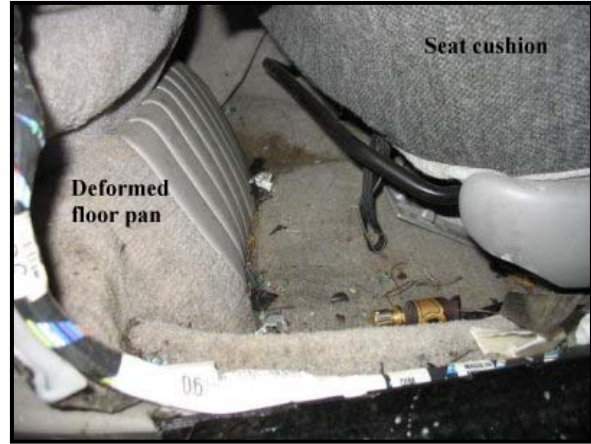
Figure 9: Floor pan intrusion. Floor mats were not present.
