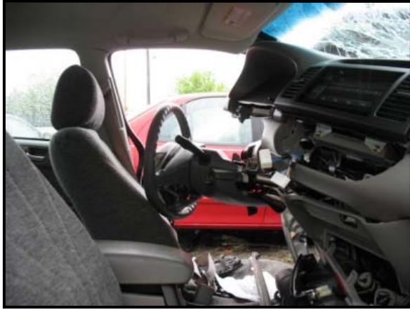
Figure 8: Right lateral view of the intruded steering wheel.
