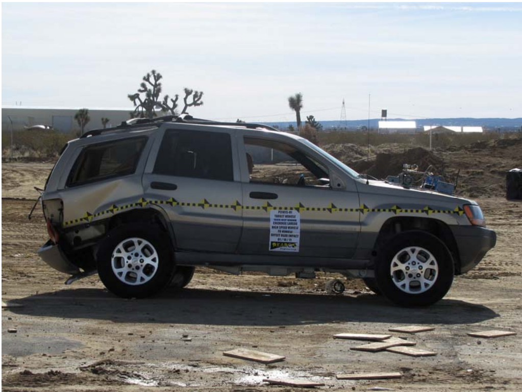
FIGURE 38. Post-Test Target Vehicle, Right Side
