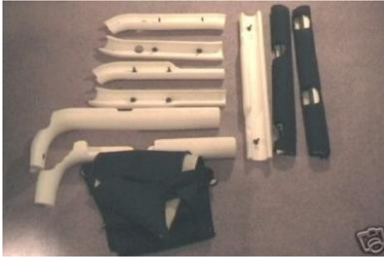
A complete set of original rollbar foam padding and the zippered cloth covers from inside a 2006 Jeep Wrangler.
