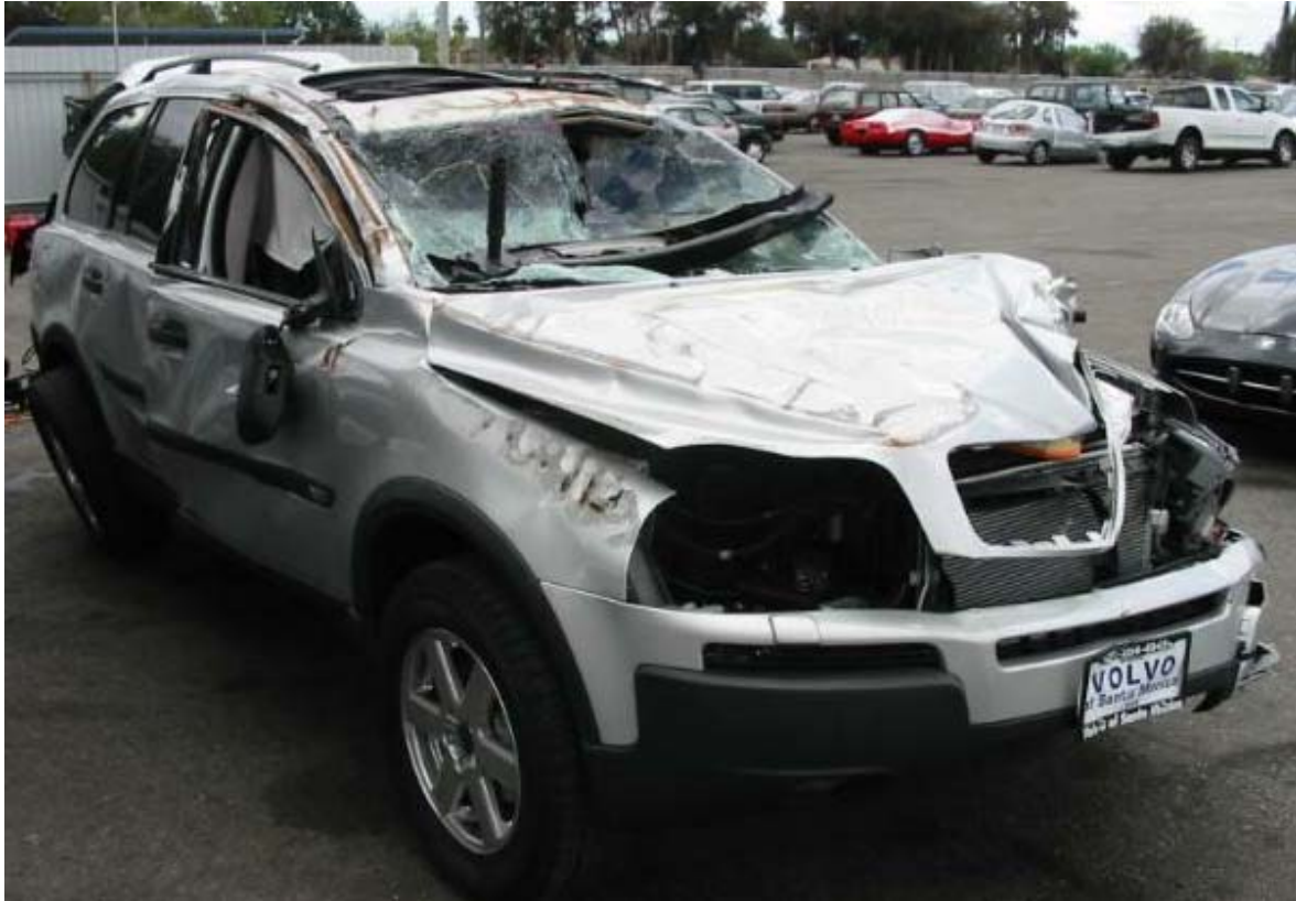
Figure 3. A Volvo XC90 involved in a rollover of 1½ rolls (NASS Case 2003-79-57).
