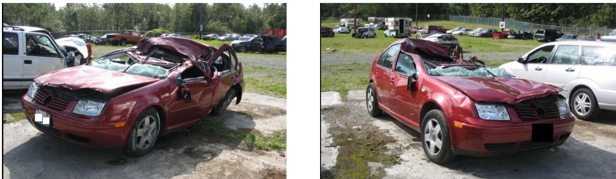
Figure 2. An example of a Class 5 NASS case where a collision (with a large tree) during a rollover was the most serious event.
