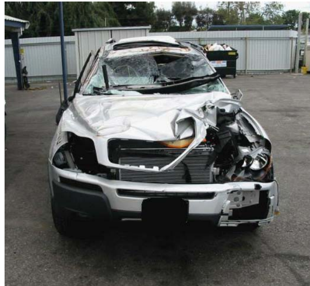
Figure 6. A Volvo XC90 with a strong roof after a rollover (NASS Case 2003-79-57).
