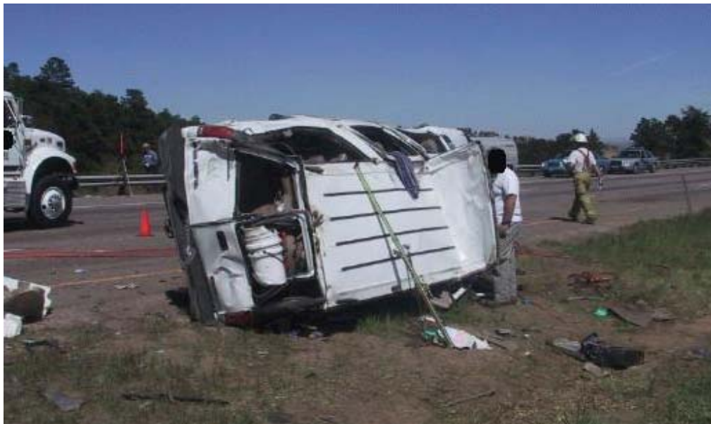
Figure 5. A 1997 Chevrolet Suburban that rolled over. The lap/shoulder belted driver suffered fatal head injuries.
