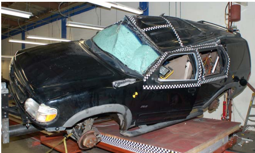
Figure 2. A 1995-2001 Ford Explorer following the second JRS test.
