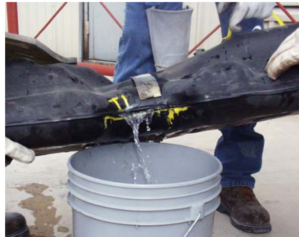
Figure 17. Seasoned “Long” Tank Post Drop Test
