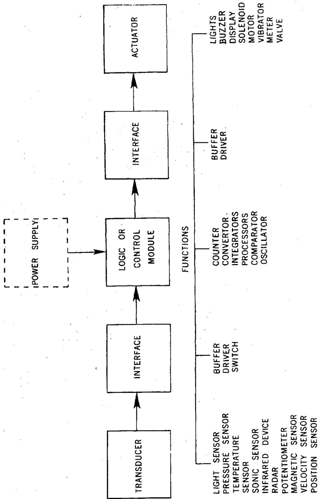
Figure 2.1 Functions and Elements of Electronic Subsystems
