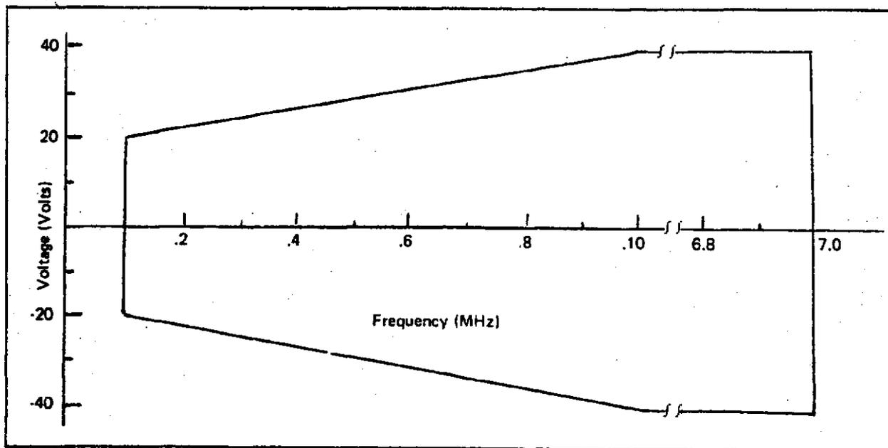
Figure 3.4 High Frequency Noise Envelope
