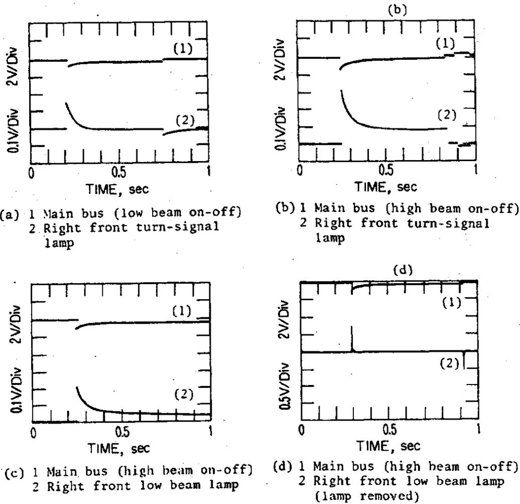
Figure 3.1 Light Switch Signals
