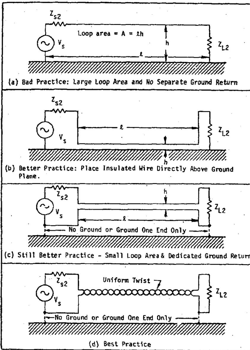
Figure 5.7 Evolution of Reducing Loop Area in Magnetically Susceptible Circuits (After White, 1973) (Courtesy Don White Consultants, Inc., Vol. 3, EMI Control Methods and Techniques.)
