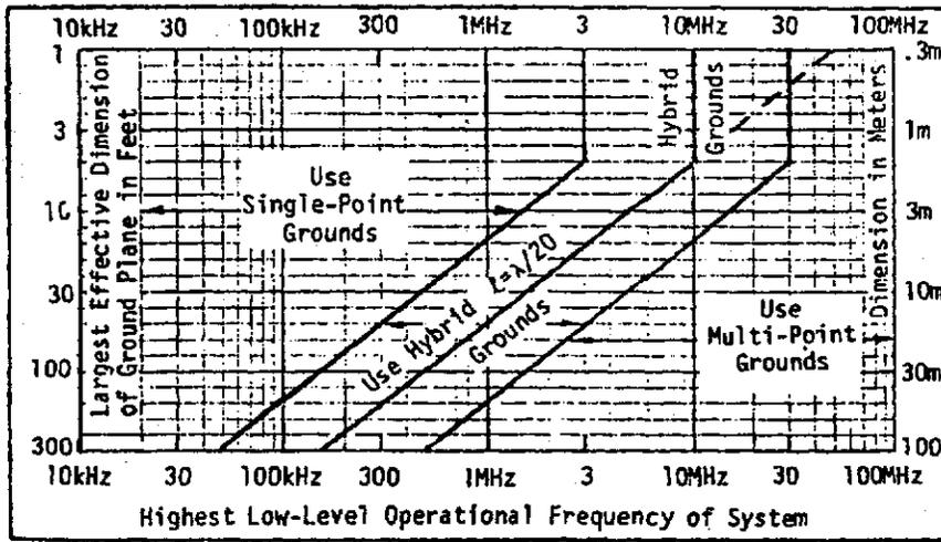
Figure 5.5 Cross-Over Regions of Single-Point vs. Multi-Point Grounding (After White, 1973) (Courtesy Don White Consultants, Inc., Germantown, MD, Vol. 3, EMI Control Methods and Techniques.)
