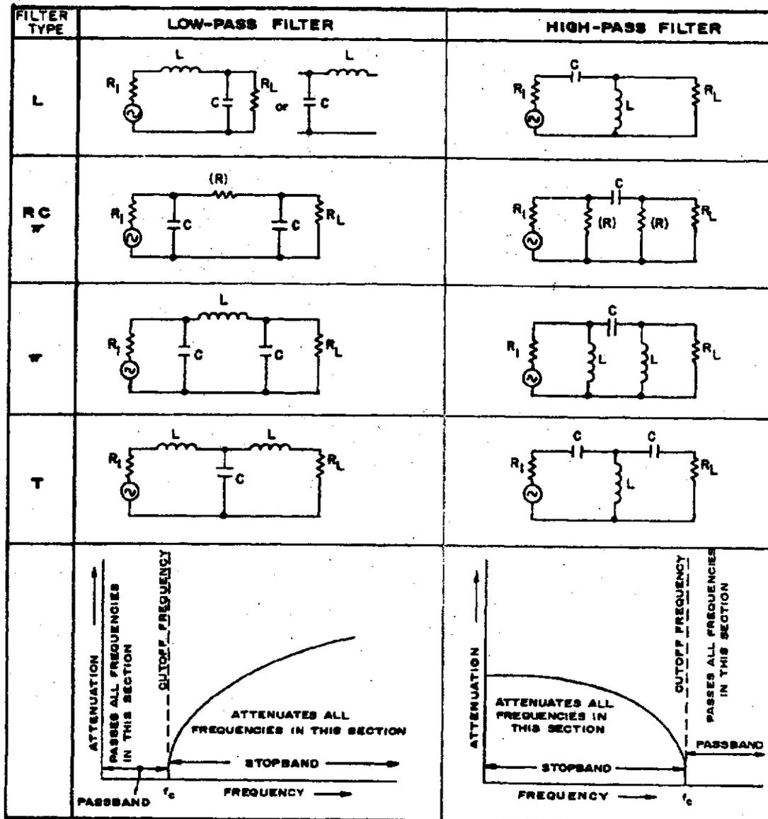
Figure 5.8 Low-Pass, High-Pass, Band-Pass, and Band-Reject Filter Configurations (After AFSC, 1973)
