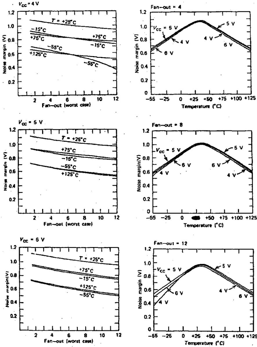
Figure 4.5 Noise Immunity as a Function of Temperature, Power-Supply Voltage, and Fan-out (After Kostopoulos, 1975) (Reprinted with permission, John Wiley and Sons, Inc., New York, NY, 1975).
