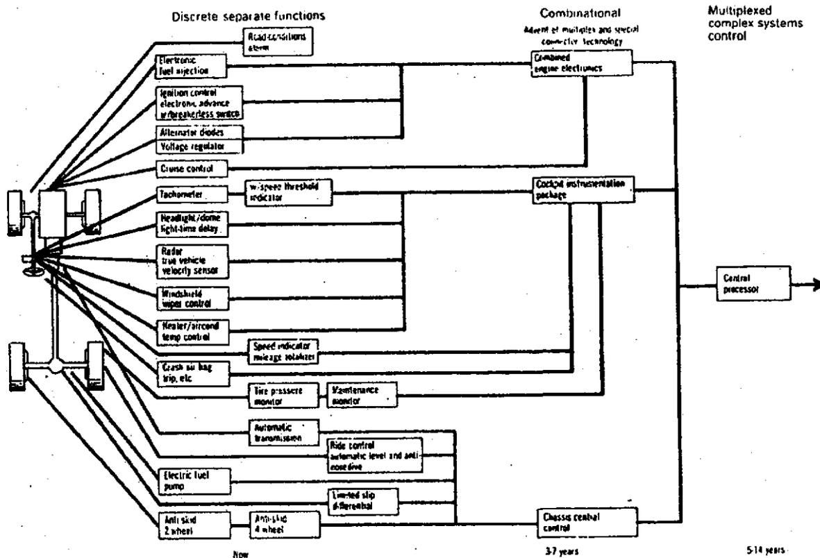
Figure 2.2 Automotive Electronic Subsystems (Hood, 1974)
