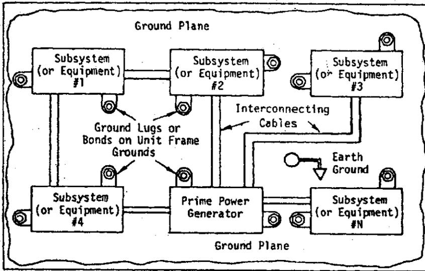
Figure 5.4 Multi-Point Grounding System (After White, 1973) (Courtesy Don White Consultants, Inc., Germantown, MD, Vol. 3, EMI Control Methods and Techniques.)
