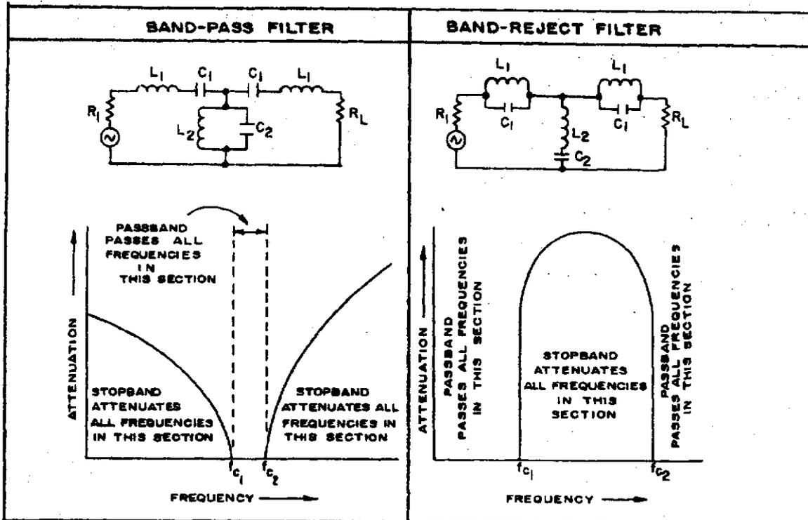
Figure 5.8 (cont.) Low-Pass, High-Pass, Band-Pass, and Band-Reject Filter Configurations (After AFSC, 1973)
