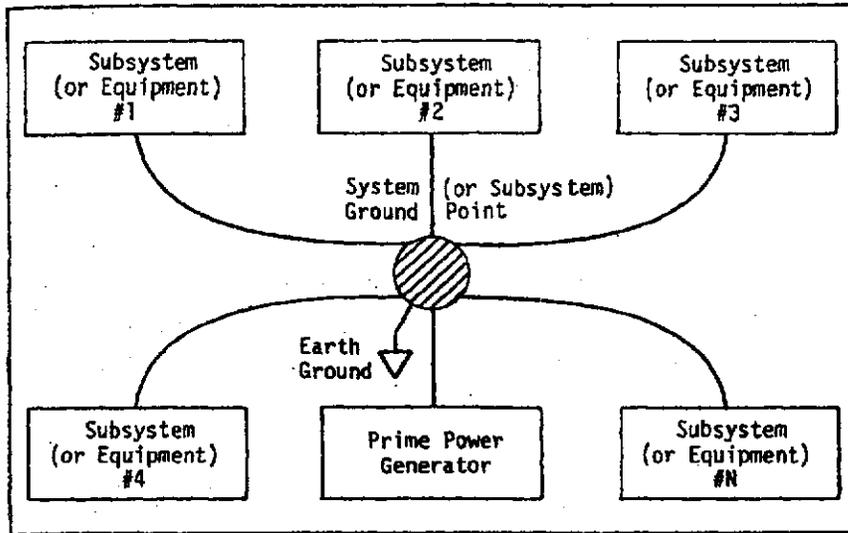
Figure 5.2 Single-Point or Star Grounding Arrangement (After White, 1973) (Courtesy Don White Consultants, Inc., Germantown, MD, Vol. 3, EMI Control Methods and Techniques.)
