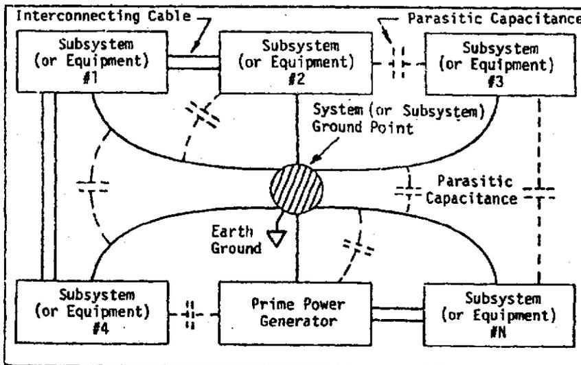
Figure 5.3 Degeneration of Single-Point Ground (After White, 1973) (Courtesy Don White Consultants, Inc., Germantown, MD, Vol. 3, EMI Control Methods and Techniques.)
