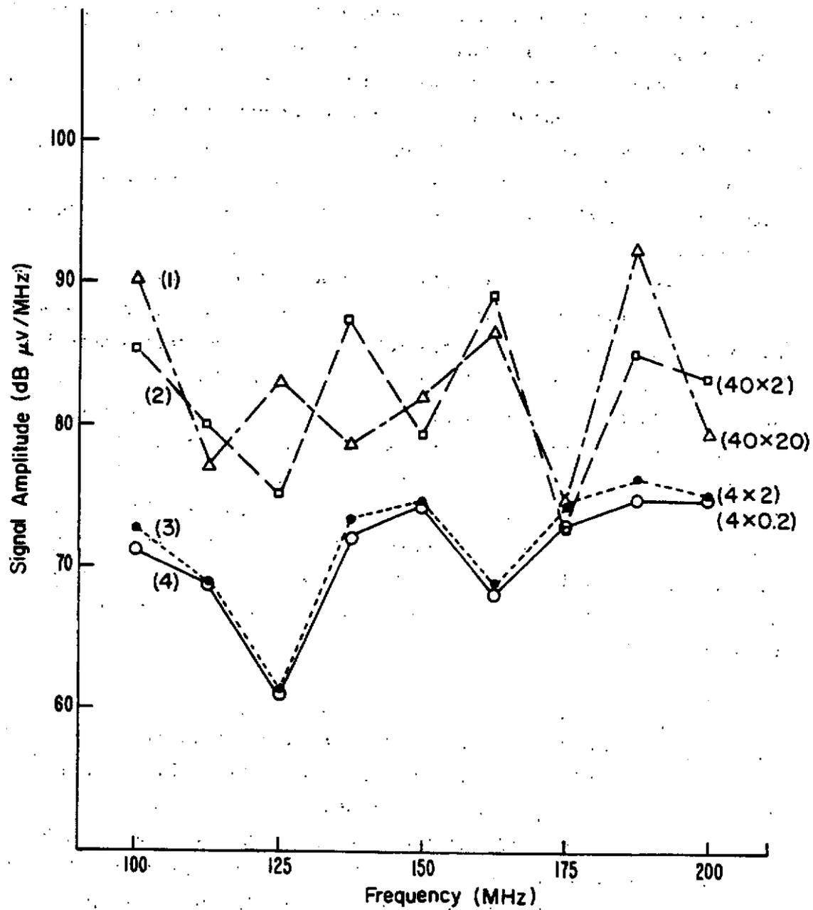
Figure 4. Signal Amplitude at a Wire Termination as a Function of Aperture Dimension. (Data points indicate coupled signal variation with frequency as a function of body shield apertures.)
