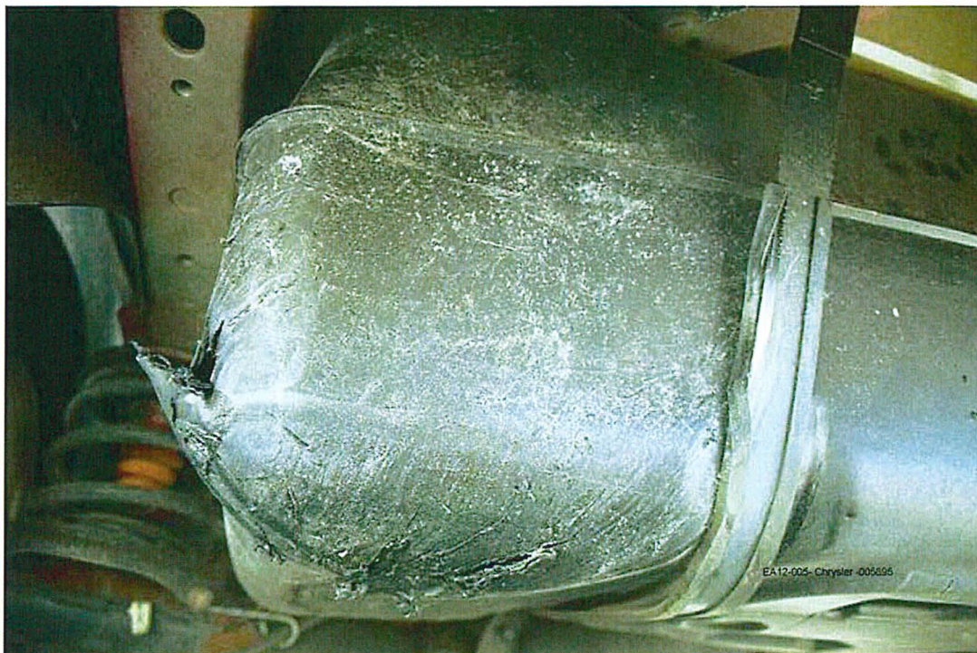
Figure 4 Rear Impact Damaged 2002 Liberty Fuel Tank.
