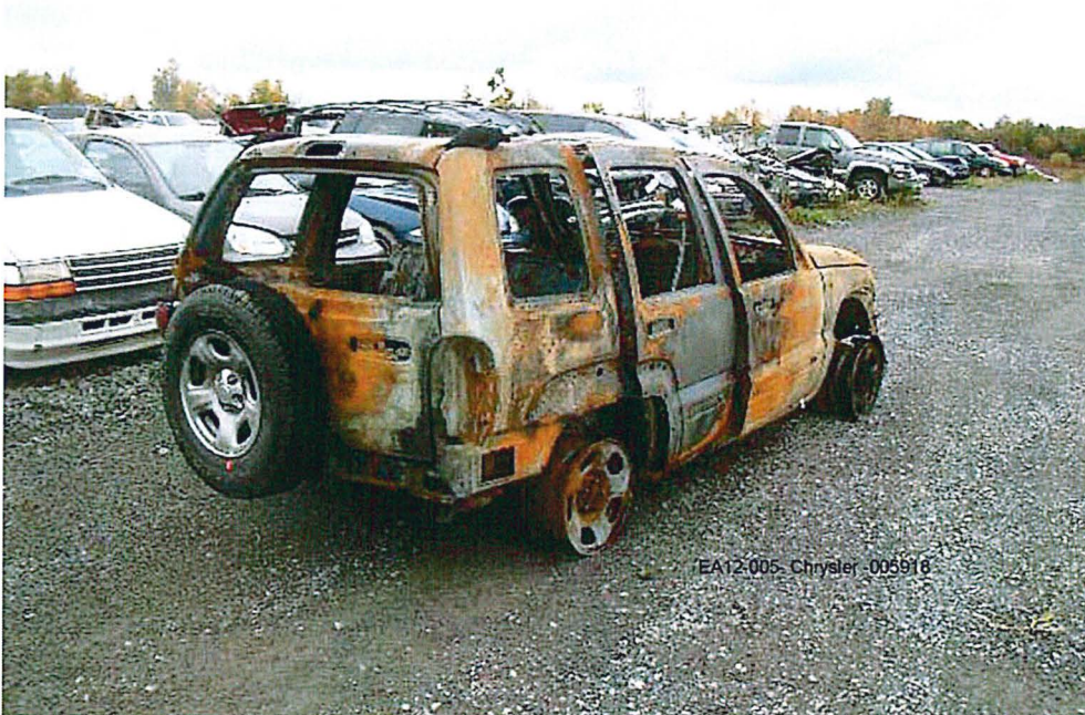
Figure 3 - Post-Crash photograph of 2004 Jeep Liberty Struck from behind by a Plymouth Neon.
