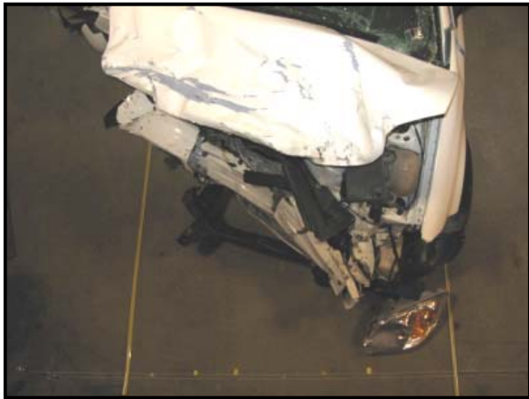
Figure 6: Overhead view of the Cobalt's frontal damage.
