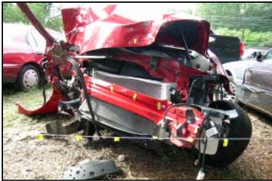
Figure 7. Damage from the 13 cm (5") tree.
