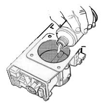
Flush the ETM bore using cleaner H on both sides of the throttle plate.
